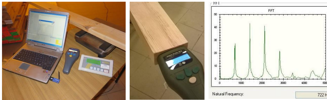
Fig. 1. An overview of the non-destructive test station with the MTG device (on the left), MTG during the determination of the MOEdyn and class C wood durability (in the centre), and a screenshot from the computer software presenting an example of the registered vibrations induced by the MTG device (on the right)
