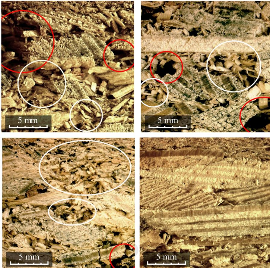
**Fig. 8.** Differentiation in the structure of chip-sawdust boards (red marks indicate empty spaces; white marks indicate spaces with sawdust).
