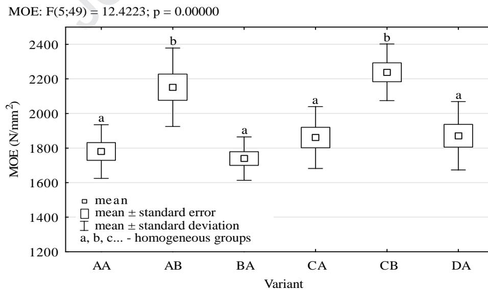
**Fig. 9.** Modulus of elasticity for bending strength of chip-sawdust boards.
