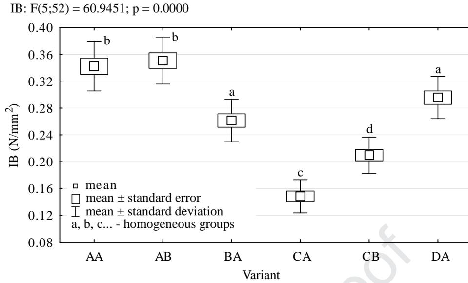
**Fig. 11.** Internal bond of chip-sawdust boards.
