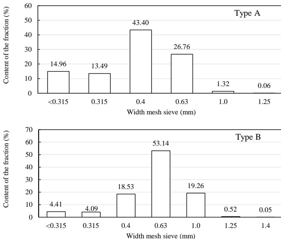
**Fig. 3.** Fractional composition of wood particles added to the outer layers of the chip-sawdust boards.
