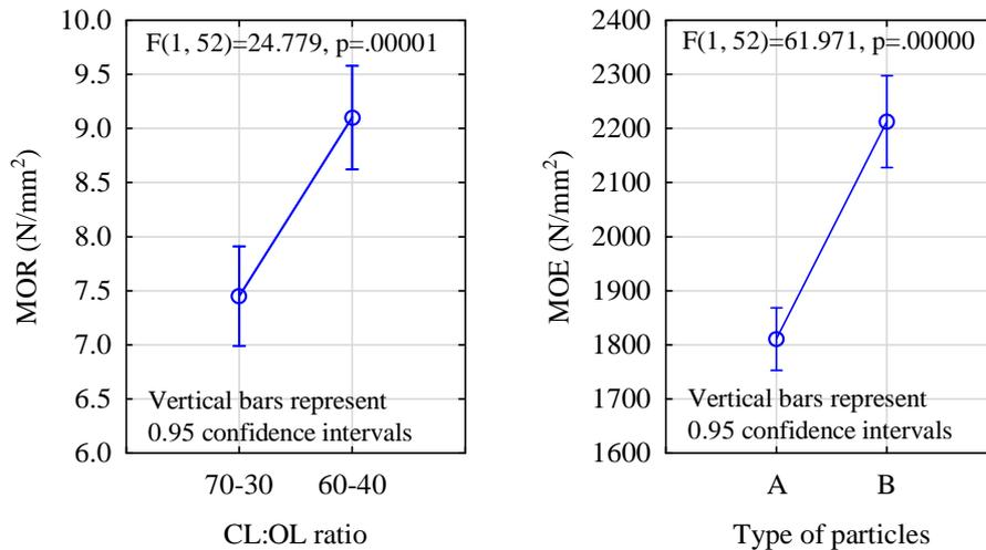
**Fig. 10.** Interaction diagram of modulus of rupture and modulus of elasticity of chip-sawdust boards depending on the analyzed factors.
