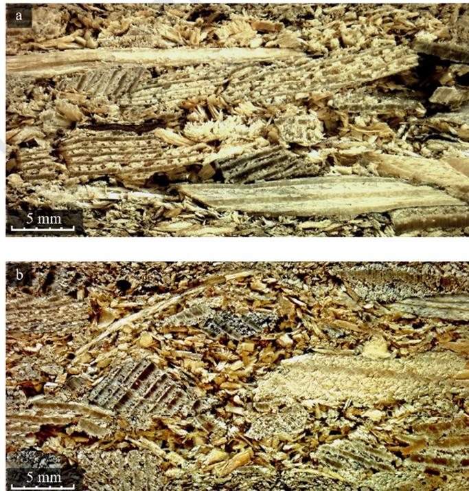
**Fig. 12.** Core layers chip – sawdust boards with chips : sawdust weight ratio: a - 70 : 30, b – 60 : 40.
