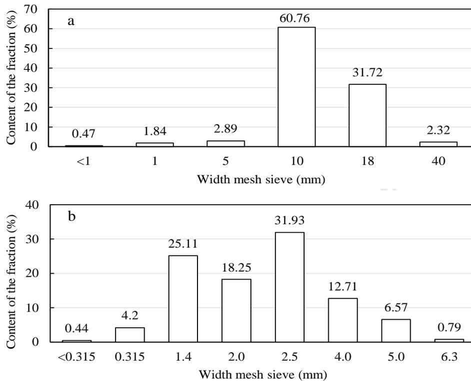
**Fig. 2.** Fractional composition of the core layer materials used in the manufacture of chip-sawdust boards: a - chips, b – sawdust.
