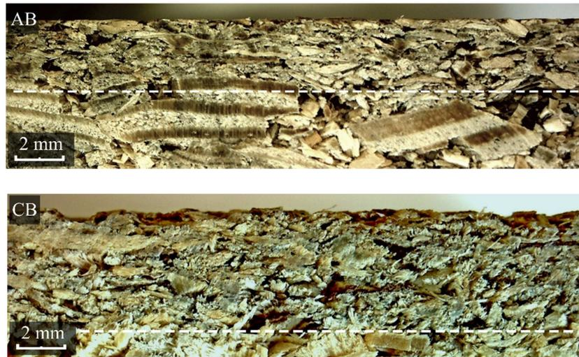
**Fig. 6.** Outer layers of chip - sawdust boards – AB and CB variant.
