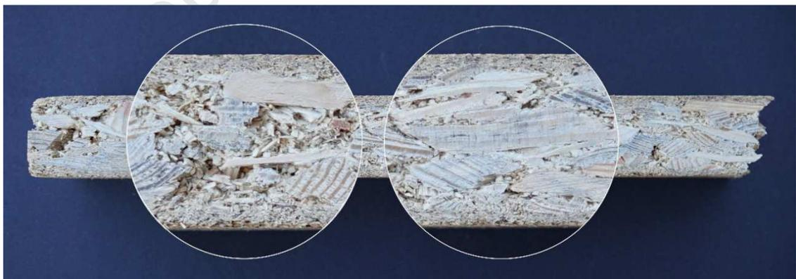
**Fig. 7.** Cross-section of a chip-sawdust board.
