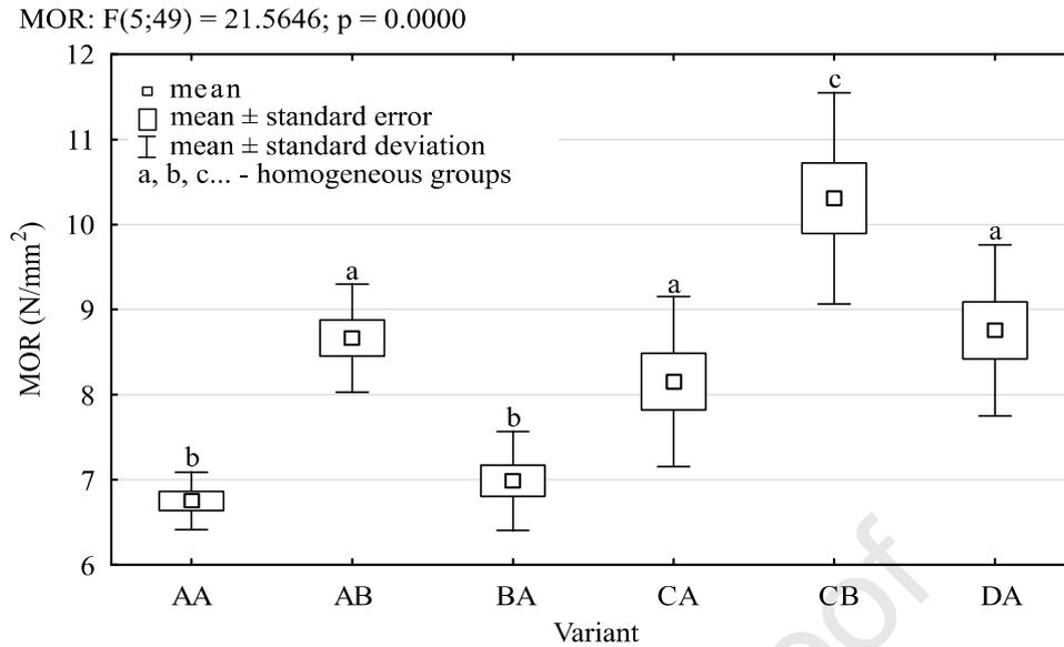
**Fig. 5.** Modulus of rupture of chip-sawdust boards.
