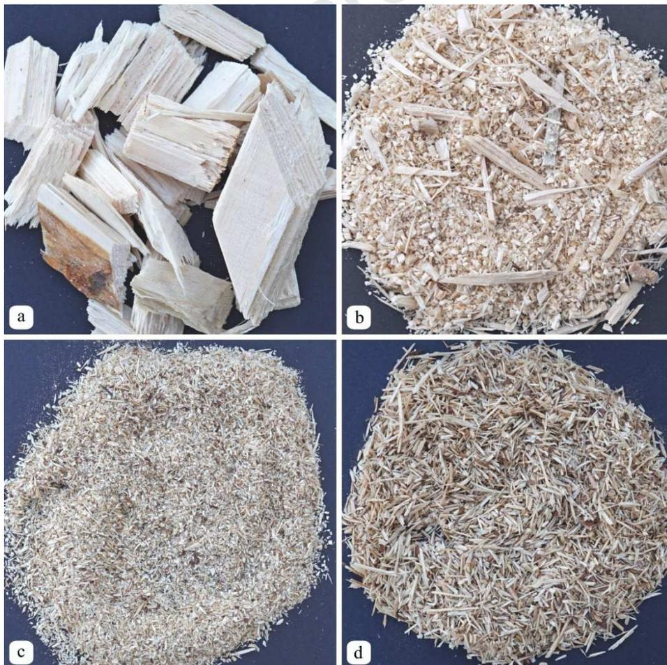
**Fig. 1.** Wood raw materials used for the production of chip-sawdust boards: a - chips; b - sawdust; c, d - particles of the outer layers, type A and B, respectively.
